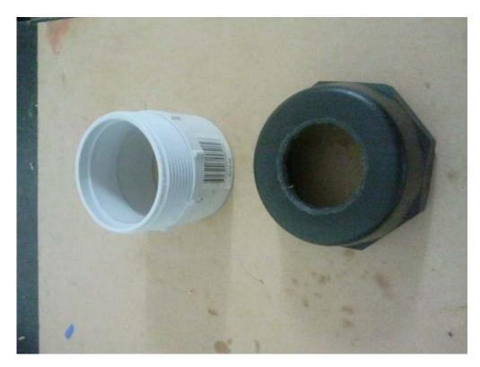
Ok now you have the hole in the cap so the plunger slides nice and smooth, fit the cap to the plunger and glue the gasket end to the plunger, you will need to glue this or it will come off in the tube. DO THIS AFTER YOU DECIDE ON THE LENGTH, you want the plunger to stop just before the Y piece.
