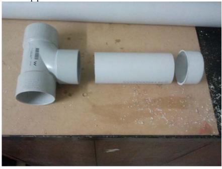
If you find that the nozzle connector won't go over the one end of the Y join, you can gently heat the end of the Y join over a flame for about 5 mins, this will soften the pipe allowing you to push the nozzle connector into position. Hold the pieces together and you should end up with a tight fit, I did not glue this as I did not want to take the Nozzle off again. It is a pain but you will get there.
