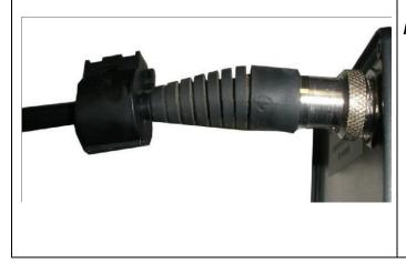
Included in the base package are 2x ferrite EMI suppressors.
