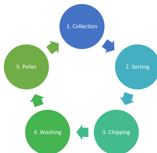
Figure 3. Overview of the plastic recycling process 1
