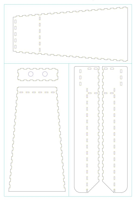
5mm acrylic (the drawings are scaled down to fit the page use the DXF file for construction)
