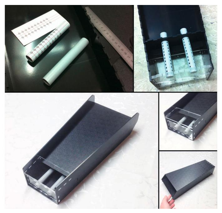
I've used 3mm ABS plastic for the corpus and 5 mm acrylic for the grizzly top and front plate to be able to see inside the trap.
