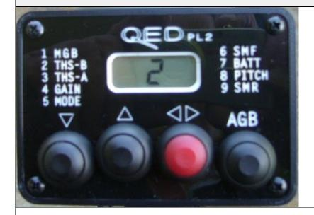
The display is an all lighting conditions 3 Digit LED Backlit LCD display.
