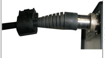
Included in the base package are 2x ferrite EMI suppressors.as required by Australian Law. One ferrite EMI suppressor needs to be fitted to the search coil plug inserting into the detectors control box for each coil intended to be used with the detector.
