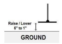
Note: Do not hit the search coil with the ground surface as this can produce unexpected results when trying to ground balance the detector.
