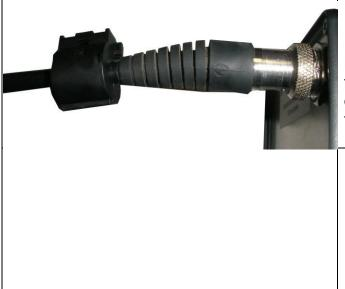
Included in the base package are 2x ferrite EMI suppressors.as required by Australian Law. One ferrite EMI suppressor needs to be fitted to the search coil plug inserting into the detectors control box for each coil intended to be used with the detector.
