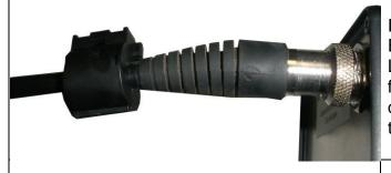
Included in the base package are 2x ferrite EMI suppressors.as required by Australian Law. One ferrite EMI suppressor needs to be fitted to the search coil plug inserting into the detectors control box for each coil intended to be used with the detector.
