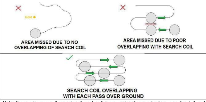
Note: If swinging a small search coil past a distance wider than each of your bodies left and right arms can result in a missed area due to poor overlapping, broader footsteps can also have the same result.
