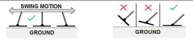
Sweep the search coil in a slow pattern as illustrated below (with the green tick) will maintain a more parallel relationship between the ground surface and the search coil; furthermore ensure the Searchcoil flows with the ground structure and make sure the search coil overlaps some of the swing area from the previous sweep over that ground.
