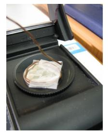
Both wires should be single conductor- none of that multiple conductor stuff is allowed. In other words, if you strip the jacket or coating and find a million little thin wires inside, that is not the stuff you need. Make it go away, and get single-conductor.
